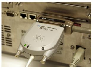
Figure 39 82357 USB-GPIB interface on a spectrophotometer
