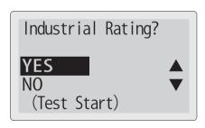
When testing the battery for industry, disconnect the all electric loads from the battery to obtain the accurate measurement.
