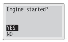
Select NO and press ← (ENTER) Key, Battery System Test Result is displayed as shown in Step ④. (judgement is done with the measured value.)
