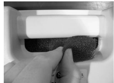
The filter is easily removed and reinserted through the gap in the back case.
