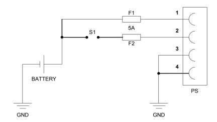
Battery (pin 1), i.e. the computer's power supply (+28 VDC) is coupled directly to the vehicle's battery (BATTERY) through a 5 A fuse (F1).
