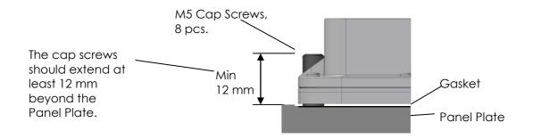
The drawing above illustrates the spacing of the eight mounting holes for panel mounting from the rear. The drawings below show unit dimension, mounting holes placement and cut out for display, buttons and indicators. For other dimensions please see the section weight and dimensions.
