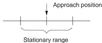
When the tolerance window for idle is exceeded, the FM 354 signals a “Stationary Range” error (see Troubleshooting, Table 11-5, Class 1/No. 12).
