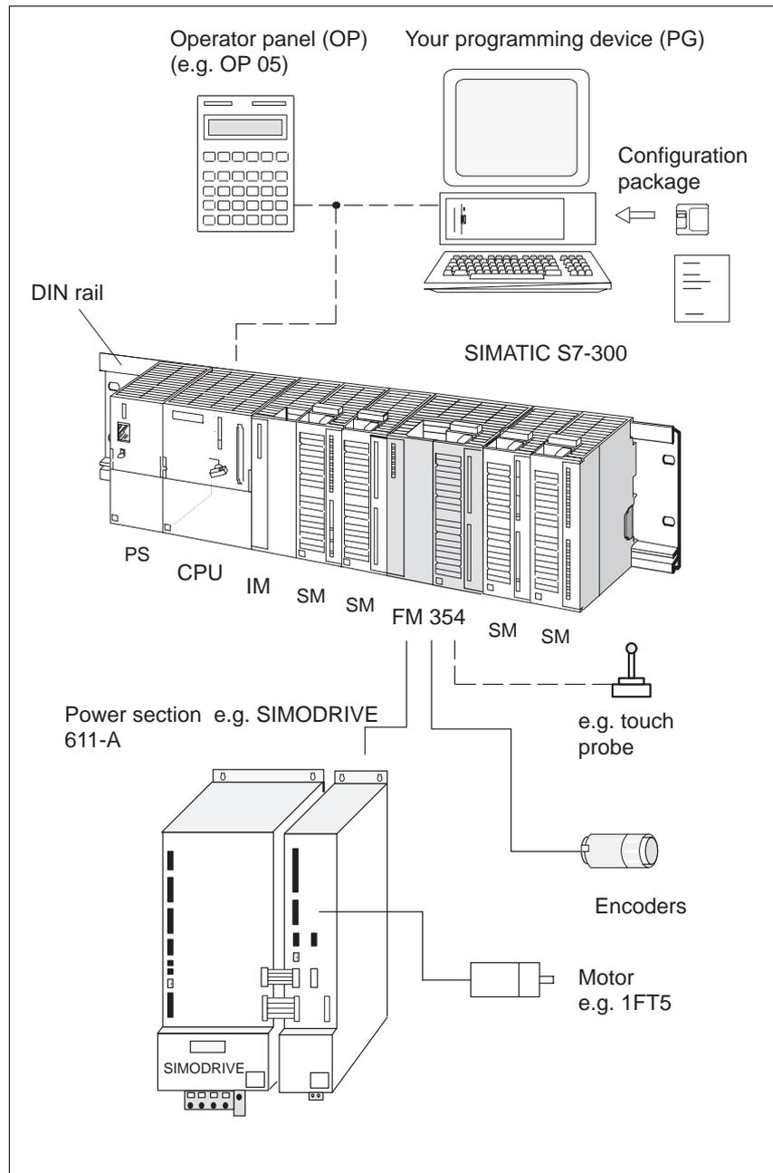
Fig. 1-2 System overview (schematic)
