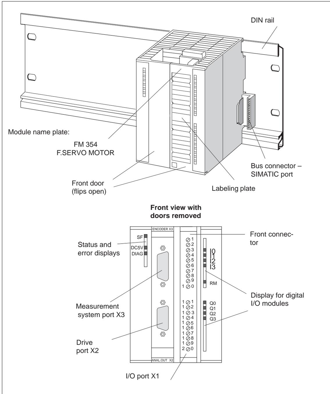
Fig. 1-4 View of the ports and front-panel elements
