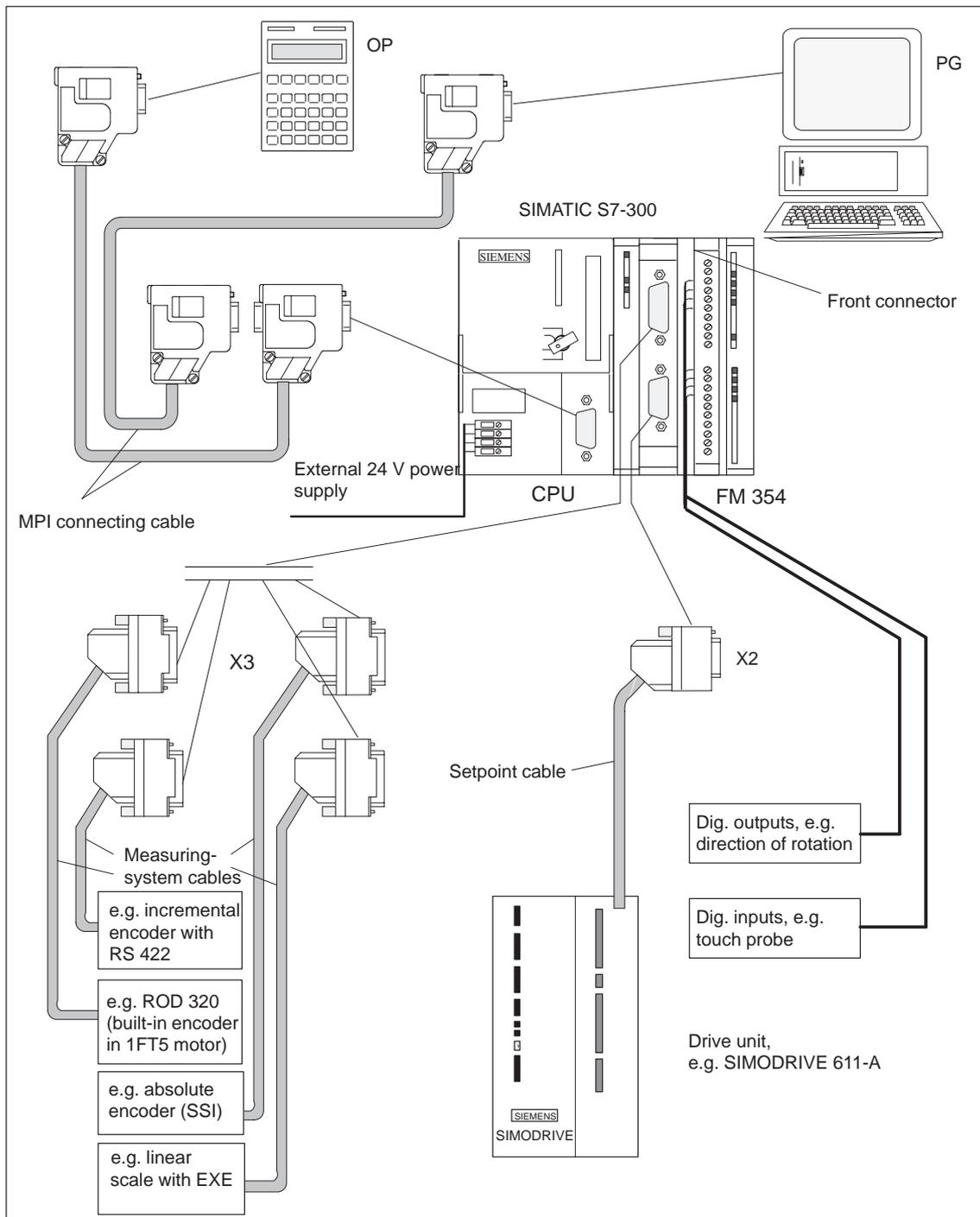
Fig. 4-1 Wiring diagram of an FM 354
