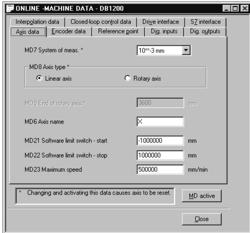
Fig. 5-4 Entering values for machine data
