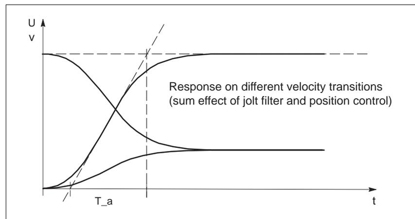
Fig. 7-13 Response on different velocity transitions (sum effect of jolt filter and position control)
