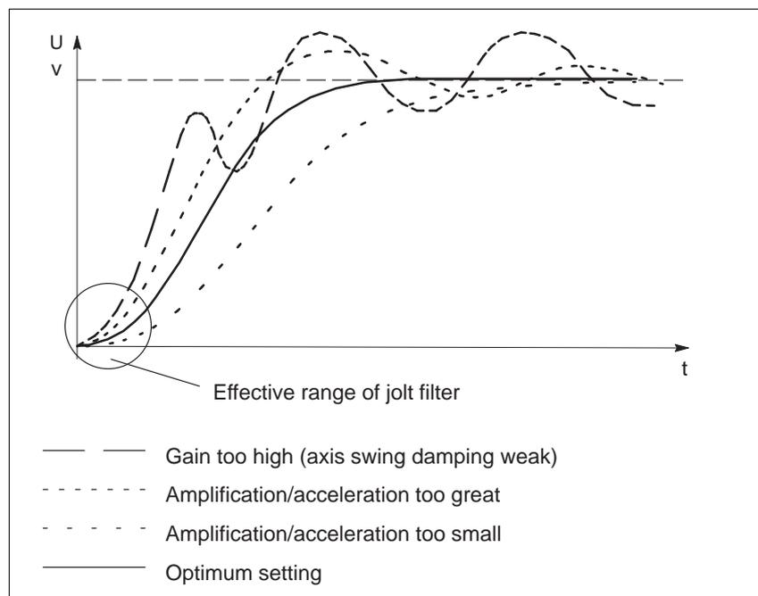
Fig. 7-12 Transition function of the position-control circuit
