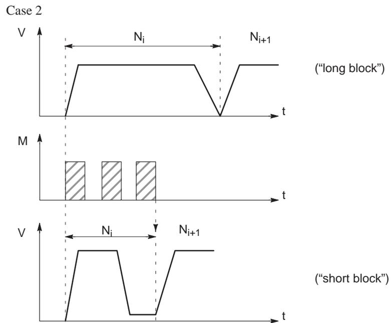
**Output of M function after positioning**
