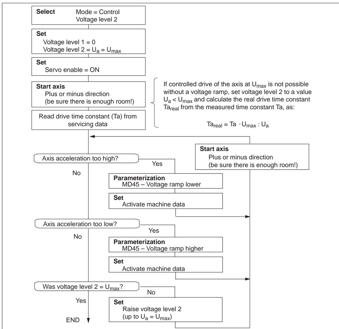
Fig. 7-7 Drive transition time and maximum voltage rise
