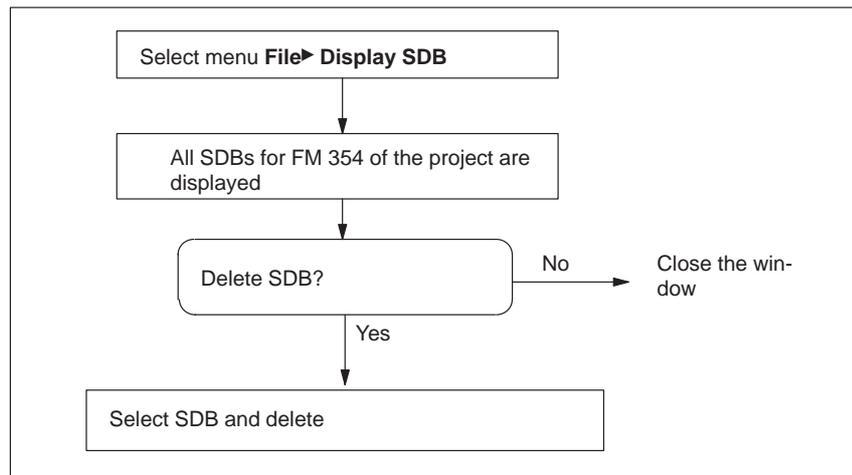
Fig. 5-9 Displaying/deleting SDB  $\geq$  1 000
