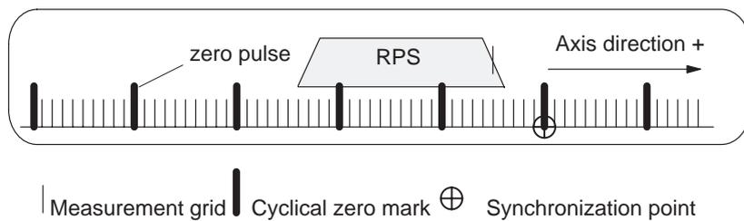
With reference to the synchronization point, the reference point can be located on the side of the lower or the higher position actual values. In the “reference point approach” operating mode the machine axis additionally traverses this distance, during its last phase of motion, once the synchronization point has been found. Consequently, the axis halts the motion, in each instance, exactly on the reference point.
