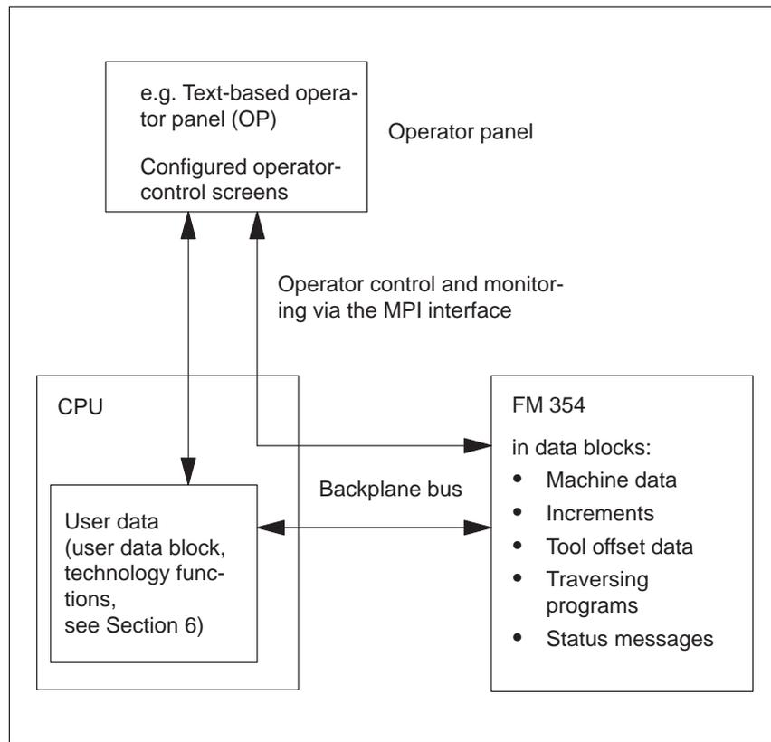
Fig. 8-1 Operator control and monitoring for the FM 354
