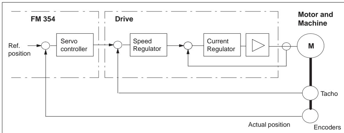
Fig. 7-10 Position control circuit
