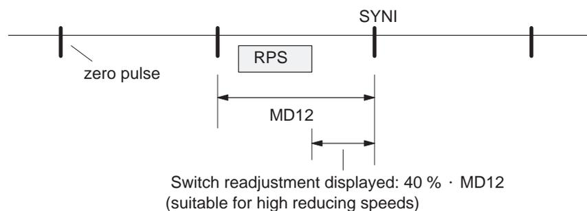
Set the referencing velocity to the highest value compatible with your requirements. It is important to be able to decelerate to the reducing velocity across the length of the reference-point switch. If this is not the case, an additional repositioning to the RPS occurs before the search phase of the synchronizing zero pulse begins. Compare the cycle of the executed traversing movements with Section 9.2.3 and optimize the referencing speed (MD28).
