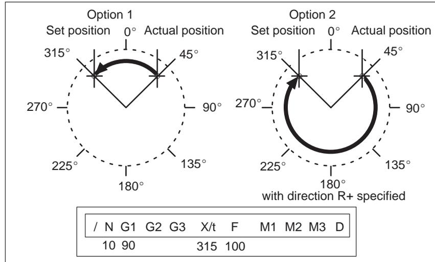
Fig. 10-3 Rotary axis
