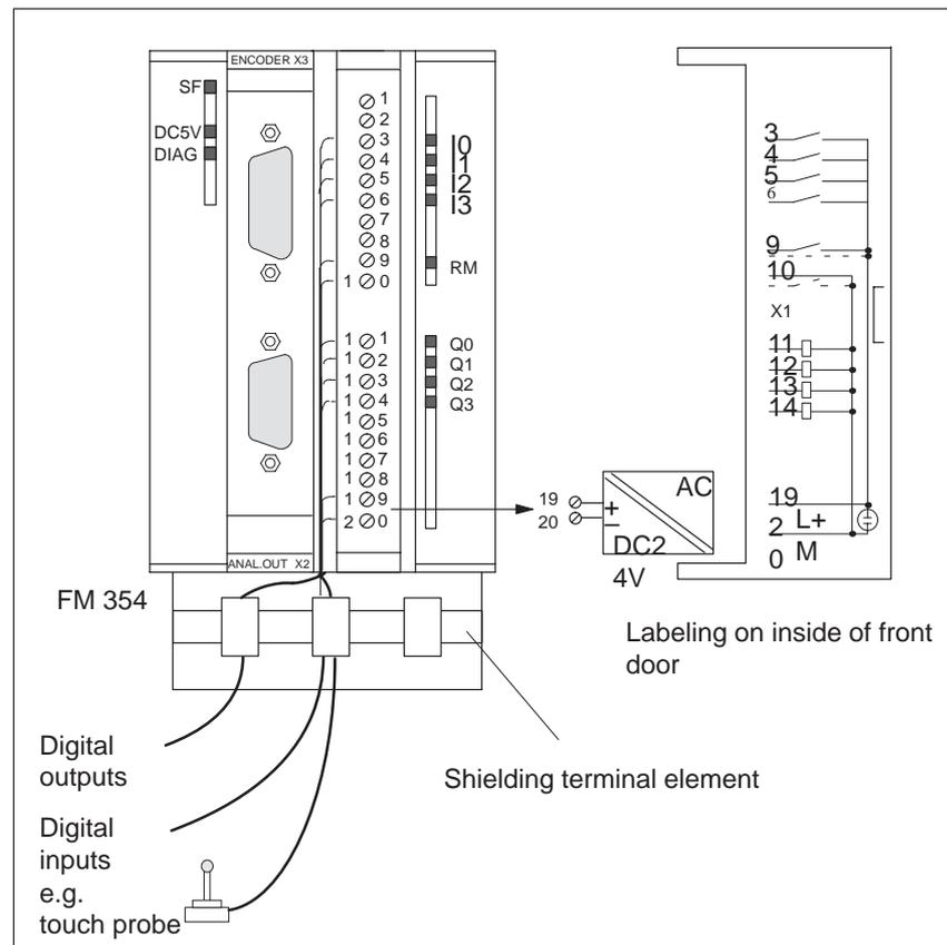
Fig. 4-9 Wiring up the front connector
