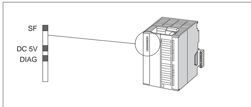
Fig. 11-2 Status and error displays of the FM 354
