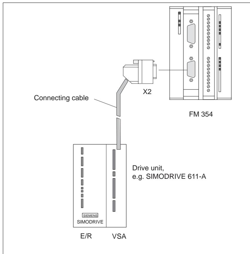
Fig. 4-3 Connecting a SIMODRIVE 611-A drive unit
