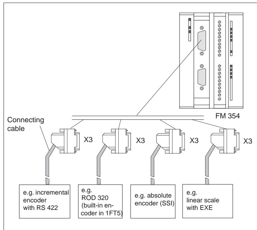
Fig. 4-5 Connecting the encoders
