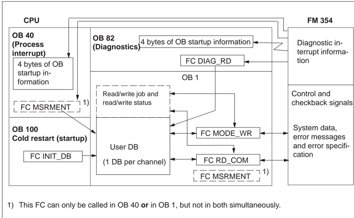
Fig. 6-2 Overview of linking the FM 354 into the user program
