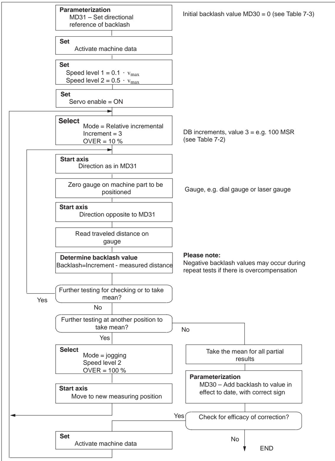
Fig. 7-15 Determination of backlash and activation of backlash compensation
