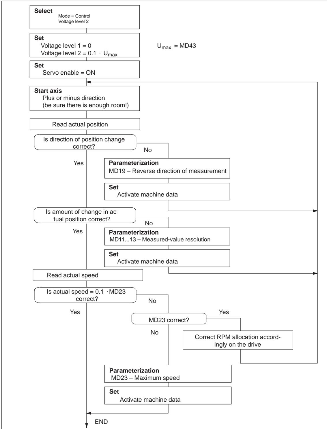
Fig. 7-6 Encoder actuation and traversing speed
