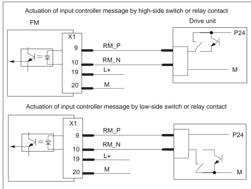
Fig. 4-8 Actuation of the input controller message, power supply from the drive unit
