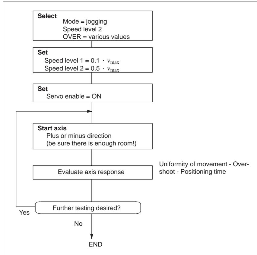
Fig. 7-11 Test movements for optimizing the servo control system
