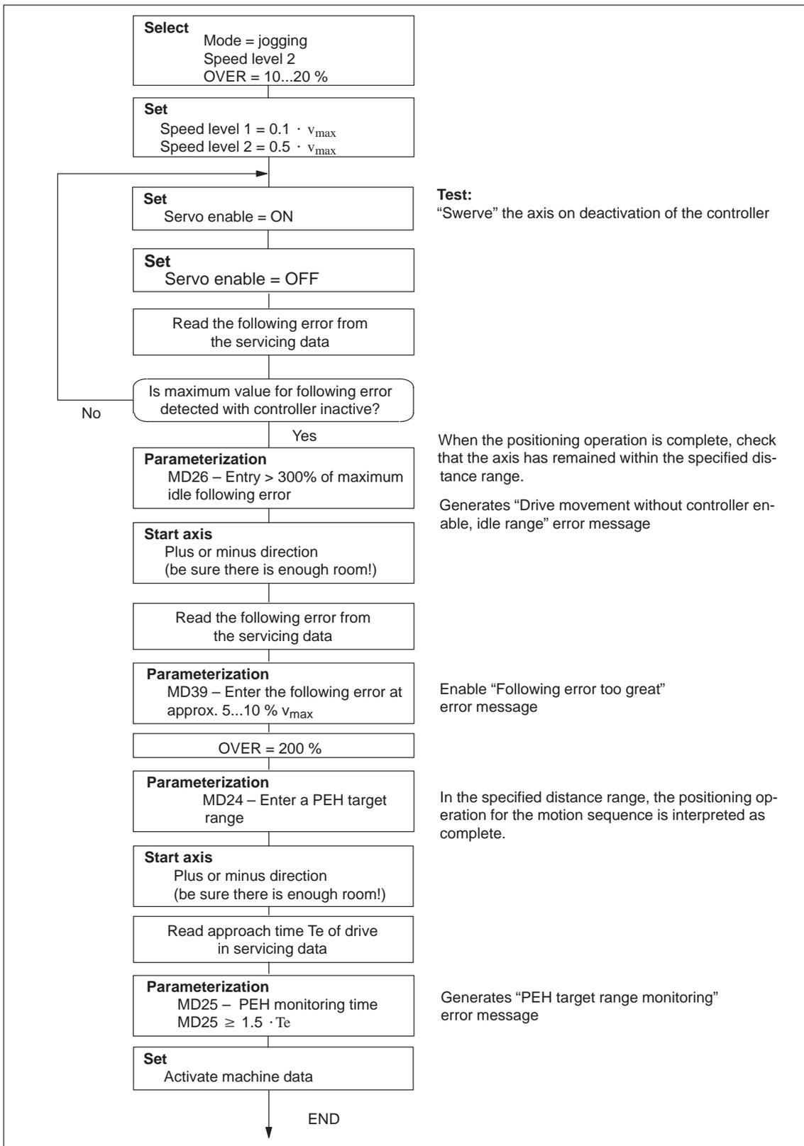
Fig. 7-14 Activation of position controller diagnostics
