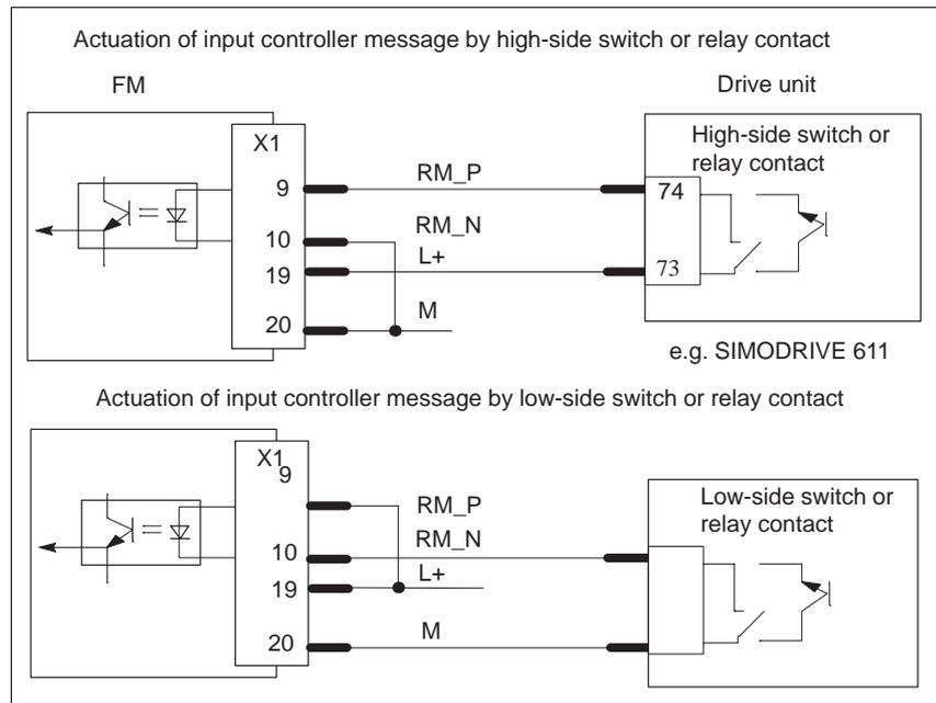
Fig. 4-7 Actuation of the input controller message, power supply from the control
