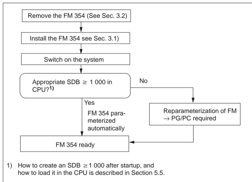
Fig. 3-1 Replacing the FM 354 with the system switched off
