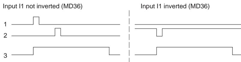
Minimum signal length at the digital input:  $\geq 2 \cdot \text{FM cycle}$
