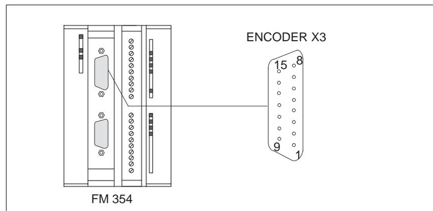
Fig. 4-4 Location of the X3 connector
