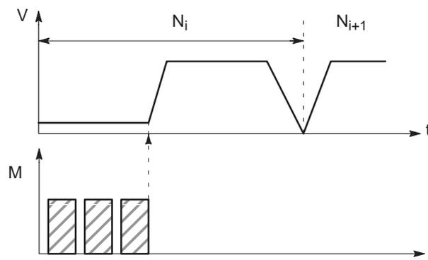
**Output of M function during positioning**
