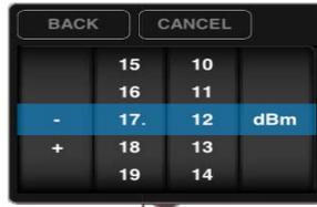
The threshold level is controlled with a bubble located on the far right of the screen. Touch and drag the bubble either up or down in order to manually change the threshold. A horizontal line and **6.00 dBm** will then appear to the right of the bubble. Also, the interface will show a color gradient using the selected colors for Min and Max.
