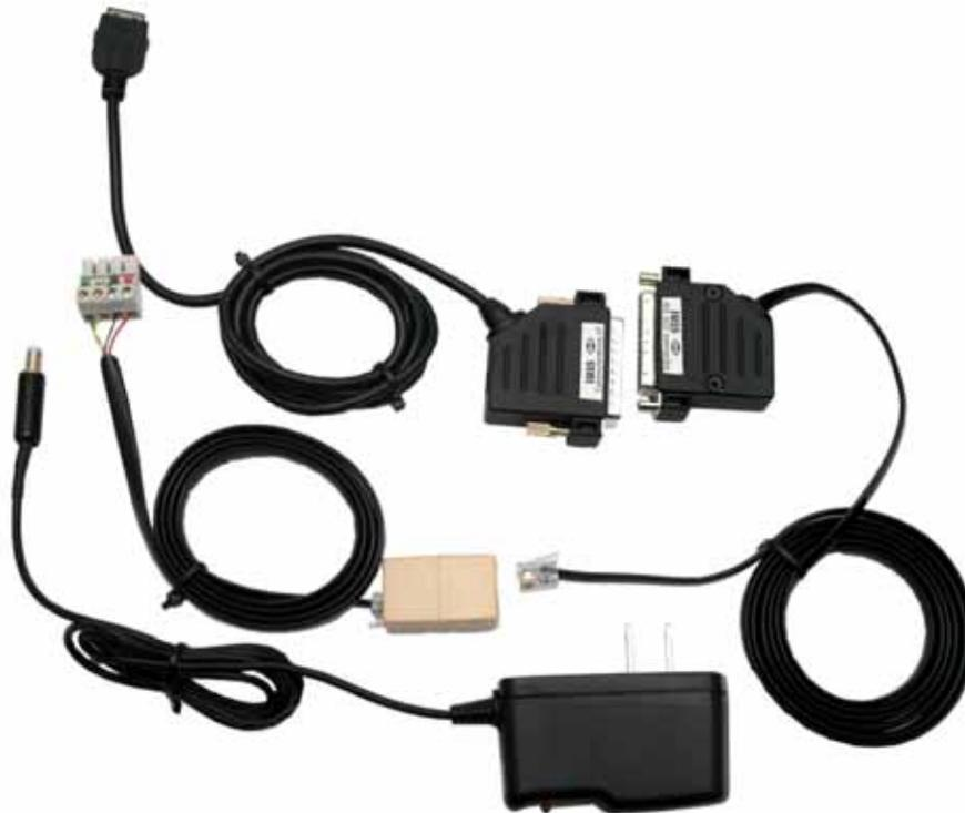
**FIGURE 12: IRIS PDA-P53x CONNECTOR INTERFACE KIT**
