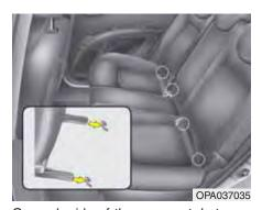
On each side of the rear seat, between the cushion and backrest, are located a pair of ISOFIX anchorage points together with a top tether mounting on the floor behind the rear seats. During the installation, the seat has to be engaged at the anchorage-points in a way you can hear it clicking (check by pulling!) and has to be fixed with the Top Tether-belt on the belonging point on the floor behind the rear seats.
