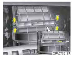
Remove the climate control air filter cover pulling out both sides of the cover.
