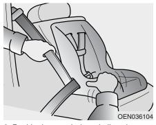
Buckle the seat belt and allow the seat belt to take up any slack. After installation of the child restraint system, try to move it in all directions to be sure the child restraint system is securely installed.
