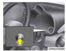
Odometer, tripmeter A or B can be selected by pressing the trip mode/reset button for less than 1 second, and then releasing.
