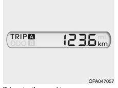
**Tripmeter (km or mi.)** TRIP A: Tripmeter A
