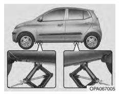
7. Place the jack at the front or rear iacking position closest to the tyre you are changing. Place the jack at the designated locations under the frame. The jacking positions are plates welded to the frame with two tabs and a raised dot to index with the jack.
