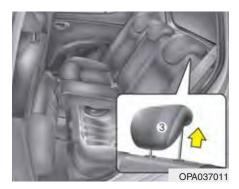
4. Remove the head restraint from the rear seatback.
