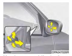
Manual remote control (if equipped) To adjust an outside mirror, move the control lever which is located at the forward inside area of the window frame.
