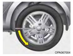
Loosen the wheel lug nuts counterclockwise one turn each, but do not remove any nut until the tyre has been raised off the ground.
