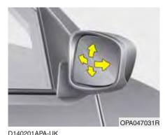
Adjusting the outside rearview mirror Manual control (if equipped) To adjust an outside mirror, move the mir-
