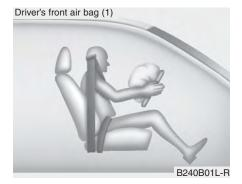
The front air bag modules are located both in the centre of the steering wheel and in the front passenger's panel above the glove box. When the SRSCM detects a sufficiently severe impact to the front of the vehicle, it will automatically deploy the front air bags.
