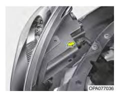
3. Disconnect the power connector from the back of the headlight assembly.
