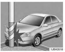
Air bags may not inflate if the vehicle collides with objects such as utility poles or trees, where the point of impact is concentrated to one area and the full force of the impact is not delivered to the sensors. C041100AEN-UK
