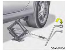
8. Insert the jack handle into the jack and turn it clockwise, raising the vehicle until the tyre just clears the ground. This measurement is approximately 1.2 in (30 mm). Before removing the wheel lug nuts, make sure the vehicle is stable and that there is no chance for movement or slippage.
