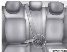
When using the rear centre seat belt, the buckle with the "CENTER" mark must be used.
