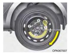
Then position the wrench as shown in the drawing and tighten the wheel nuts. Be sure the socket is seated completely over the nut. Do not stand on the wrench handle or use an extension pipe over the wrench handle. Go around the wheel tightening every other nut until they are all tight. Then double-check each nut for tightness. After changing wheels, have a HYUNDAI authorised repairer tighten the wheel nuts to their proper torque as soon as possible.
