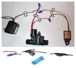
wire ends. . Connect wires as shown in the diagram above and table below using wire nuts provided. Bend wire nut connection flat to length of wire and wrap with self-adhering tape making sure to create a proper watertight seal. Apply a liquid electrical sealant (available at most hardware stores) to each connection. We recommend that the unit be tested before weatherproofing the connectors.
