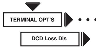
The AT\*CD (DCD Loss Dis) command determines how long the modem waits before it disconnects due to loss of carrier (DCD). If the S10 setting is selected and set to 255 or Off, the modem attempts to retrain immediately.
