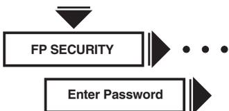
To unlock a password-protected modem and gain access to all modem functions, use the AT\*PNxxxx command. xxxx represents the password, which must be entered with the command.
