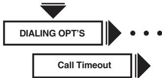
The AT\*TT (Call Timeout) command determines how long the modem waits from the time it completes dialing to the time it detects answer-back tone from the remote modem. If the modem does not receive answer-back tone from the remote modem within a specified time, the modem disconnects. The setting of this option also affects the “R” dial modifier. See **Section 8.4** for a description of dial modifiers.
