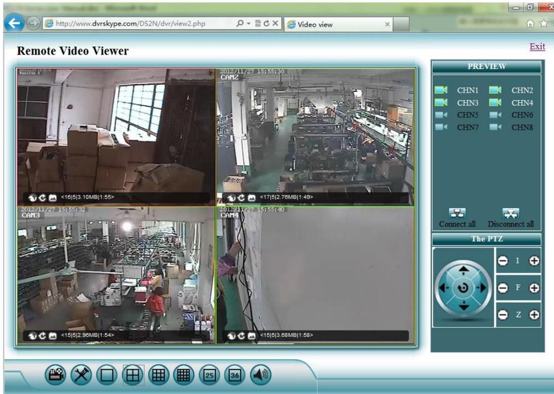
Open preview:In preview window,click left mouse,choose target channel, (If channel frame is red,means select). In channel on/off table,click left mouse,can open or close that channel video, such as:
