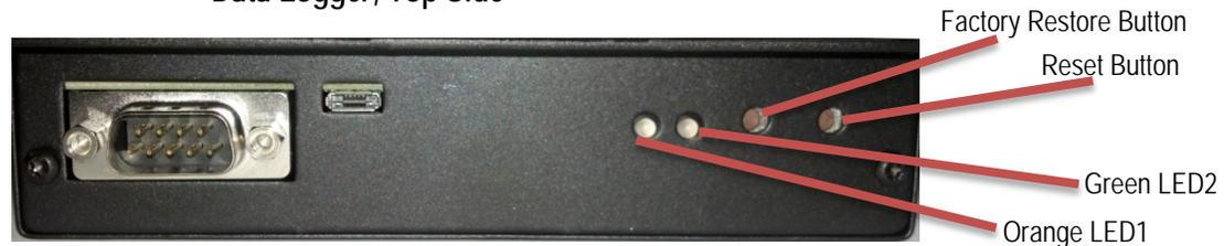
Checking the status LEDs on the logger is the first thing to do when troubleshooting a logger. A solid orange LED (or no LEDs lit when powered) is an indication that the logger is not running properly and may need replacement if the problem persists.
