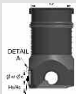
Detail of lipped joint mounted with silicone on a riser.
