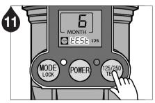
Press the TEST button for 2 seconds to run a test cycle and check for proper operation of the unit.
