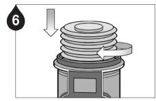
Carefully screw the grease pouch in by turning clockwise. Do not over tighten.
