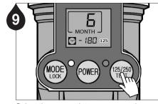
Select the appropriate grease pouch capacity by pressing the 125/250/TEST button.
