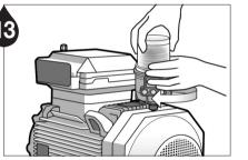
Install the Pulsarlube M unit on the lube point. When the selected dispensing period has completed, replace the unit with the Service Pack according to step #3~7.
