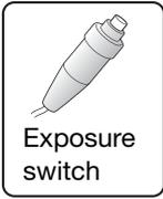
Confirm that the **Ready** indicator appears in the system status bar, and then press and hold the exposure switch of the X-ray generator.
