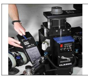
The Dolly's power is supplied by two batteries with 24 V each.
