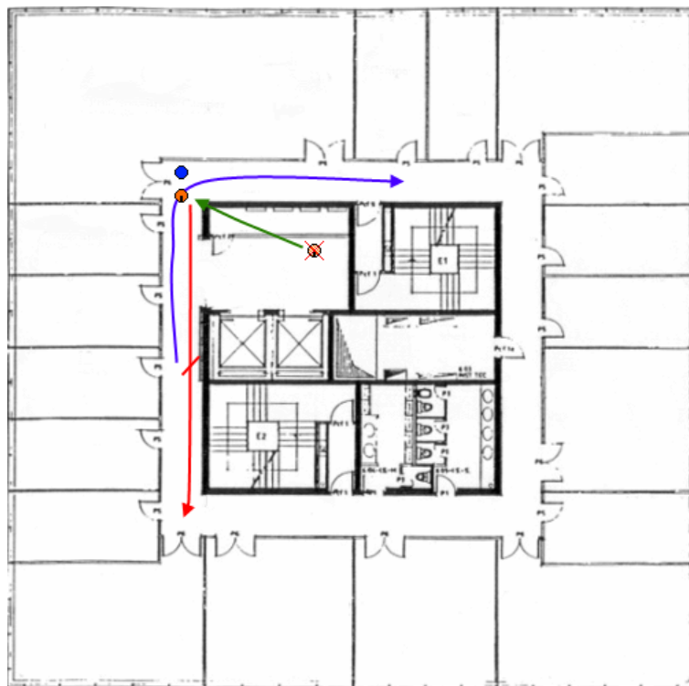
Figure 8.2: Graphic representation of the demonstration test scenario. The blue, orange, and crossed circles represent the user and robot initial positions, and the position where the Robot initially assumes to be located; the green, red, and blue arrows represent the user redefinition of the Robot's position, the first trajectory defined by the user, and the last Robot's course, which starts where the user interrupted the Robot's previous course.
