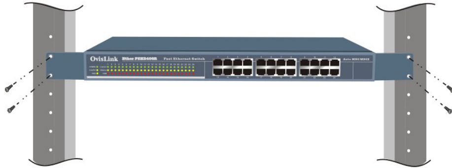
Fig. 3-2 Attaching the Switch to a 19-inch rack
