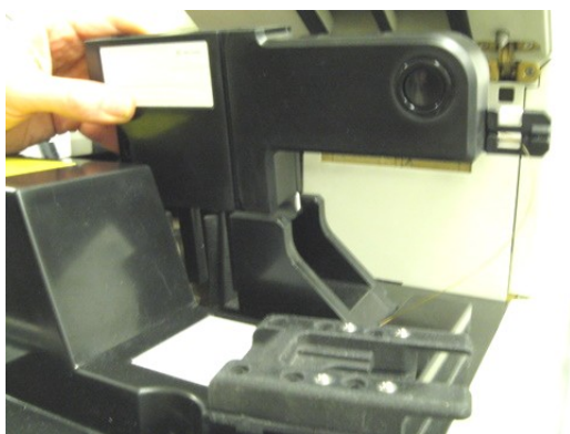
Figure 8. Load Agilent cassette into HP3D, ensuring that the sample inlet capillary finds the guide hole. To relieve tension on capillary, temporarily place the cartridge on oven surface. For more information refer to your HP3D user's manual.
