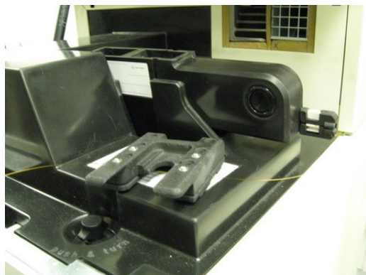
Figure 10. Lock the cassette in place. The ActiPix cartridge is now ready to be inserted.
