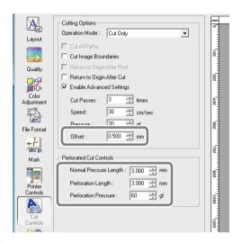
Note the following points when performing the above output operation as using the normal perforated cut.
