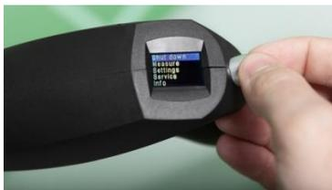
**Note!** For a more accurate leak detection it is recommended to rest the SniffIT X1® in measuring mode for approximately 10 minutes. This way the sniffer stabilizes against the environment.
