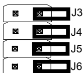
Figure 31: Intellicon-6+2 - J3, J4, J5, J6 factory settings
