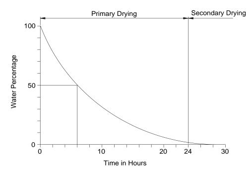
The drying time depends heavily on the vacuum level. The nearer the vacuum to the solidification point in accordance with the vapor pressure curve the shorter the drying time.
