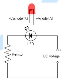
Also we must observe the position of montage of the LED, due to that has positive where (cathode) will solder the resistor connecting them to the GND of the connector that use the plate (J2 or P2) and negative (anode) we will connect to an exit of the IOCard Master. On the LED we will be able to easily distinguish it for two characteristic, in the case of the cathode is more short and also in the inside of the plastic it is seen that the foot is extended towards the side of the anode.
