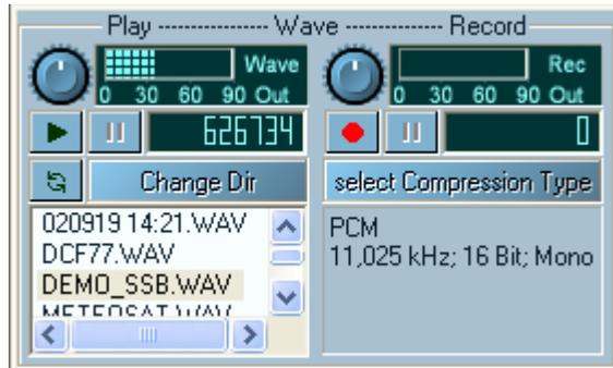
The signal recorder is used for recording or playing back signals.
