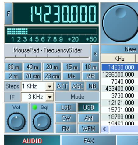
The main window includes the most important control elements for controlling the radio. You should be familiar with these functions. Your radio may not support/have all functions. Frequencies can be entered or dialed up and down by clicking the tuning knob on the left for down or the right for up. The **step** size is determined from a drop down menu when you click the button.
