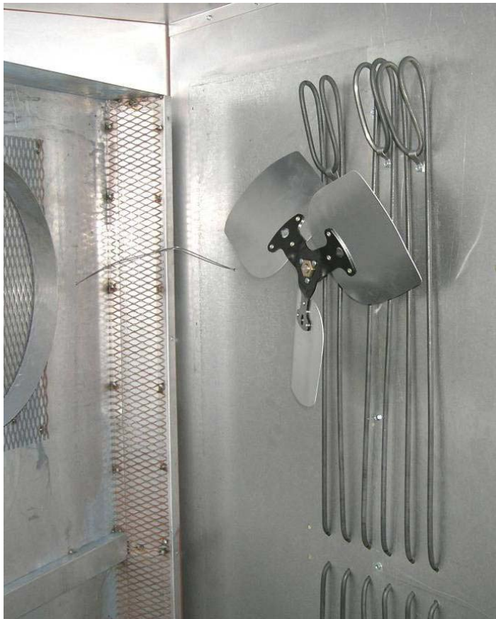
FAN AND HEATER BANK
