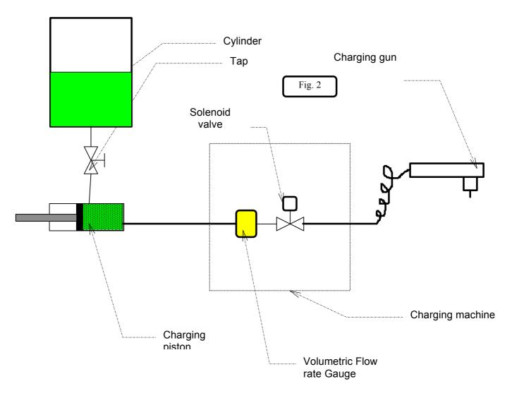
The charging piston compresses the refrigerant to a max P of 20 bar-r, thus favouring the re-condensation of any flash vapour that may have formed during transit through the line between the tank and cylinder: consider fig. 1) in which the saturated liquid (left-hand point on curve) undergoing slight pressure drops "enters" into the tank generating flash vapour and ultimately a liquid-vapour mixture.
