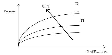
The release of refrigerant tends to cool the oil and hence oppose the release itself. For this reason, it is advisable to switch on the crankcase heating elements, if available, during the evacuation process.
