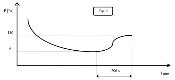
The figure represents a vacuum cycle and an optimal subsequent pressure rise for the refrigeration devices we manufacture.
