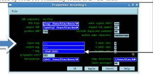
Run the scenario to generate the SEF equivalent of the sio85.evcd file. We'll name it "in.sef" for reference later when we describe automatic timing and pattern extraction from it.
