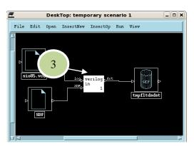
Change "make signal defn?" to YES to tell TDS to generate the Signal Definition File automatically.
