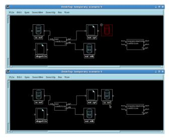
Step 5. A copy of in.sef is placed. This is the same as the first in.sef, but it is placed here for easy wiring it up to the sequencematch's wave-source (wsrc) port.
