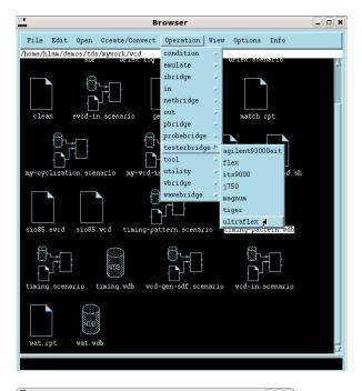
Step 2. When the ultraflex testerbridge scenario pops up, select run-> scenario and the testerbridge will generate Ultraflex tester files in the specifed "./output" directory.
