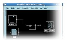
Move the "SDF" text file icon to the right and connect "verilog-in" operation up to it.
