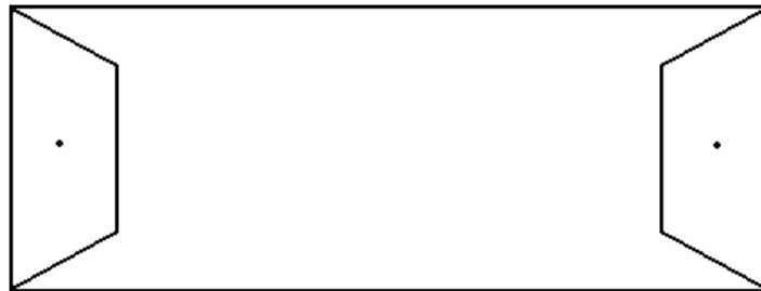
Figure 3: Diagram of a PA sample with PE grips
