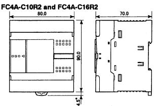
\* 8.5 mm when the clamp is pulled out.
