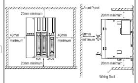
Always mount the slim type CPU modules horizontally on a vertical plane as shown above. Any other mounting directions are not allowed.
