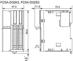
8.5 mm when the clamp is pulled out.
