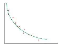
The quality of the custom calibration is (partly) based on the quality of the best-fit approximation. This, in turn, depends on the number of data points that are available. **More data is better.** If you have only a few data points then the calibration will not be reliable.
