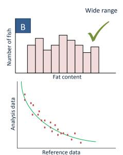
Remember, a calibration is the relationship between sensor measurements and fat content across the whole range of possible fat content values for the target fish.
