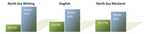
Since the ratio of fat to water can change for different fish, the Fatmeter needs to know how to relate the fat content to the measured water content. The relationship is called a **calibration**.
