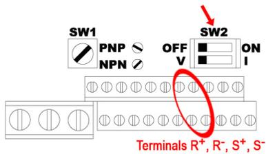
**IMPULSE®•P3 Series 2:** DIP switch SW2 is located above the control terminals, as shown to the left.
