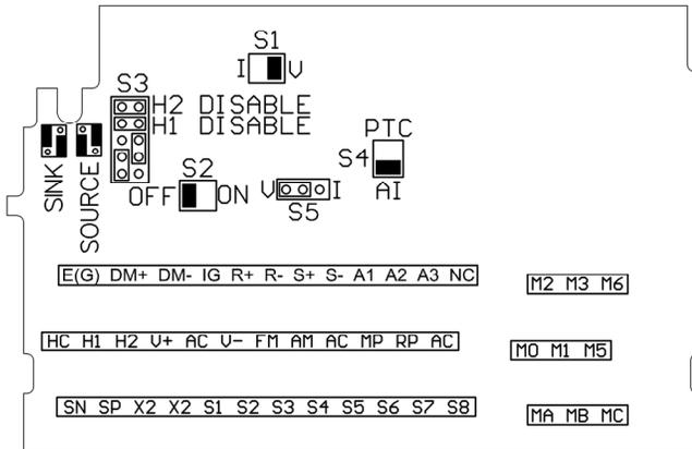
**IMPULSE®•G+/VG+ Series 4:** DIP switch S2 is located on the interface board, as shown to the left.
