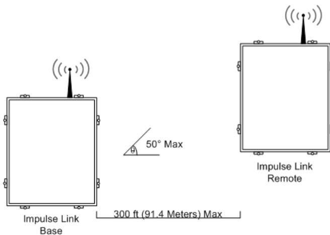
The base and remote units should be mounted on a flat, non-flammable vertical surface using four mounting screws. Line of sight should be maintained from both the remote unit's and base unit's antennas to avoid communication dropouts.
