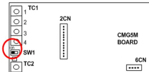
**IMPULSE®•G+/VG+ Series 2:** DIP switch SW1 is found on the left side of the CMG5M RS485 option card.
