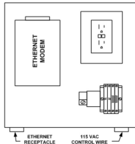
At the bottom right of the Base Unit enclosure is a cable grip for running the 115V control power wiring. The Ethernet receptacle is built in to the bottom left of the enclosure. Ethernet and control power wiring should never be run together.
