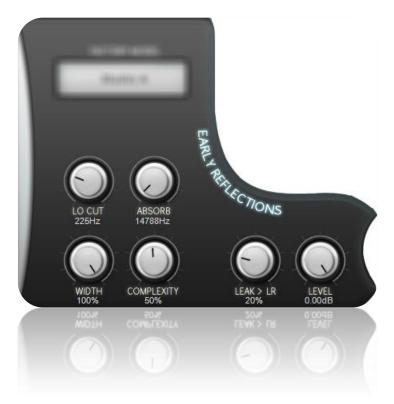
**LO CUT** controls a high pass filter which should help to avoid low frequencies to expend too much.
