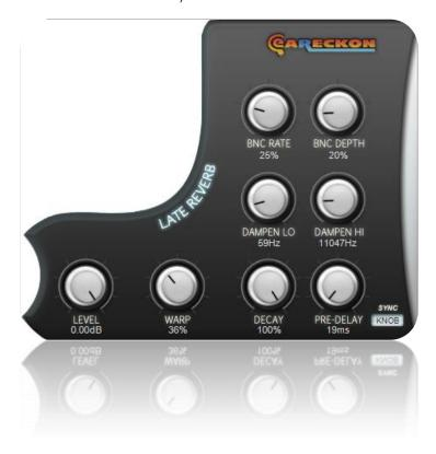
**DAMPEN LO** controls a high pass filter which should help to avoid low frequencies to diffuse too much.
