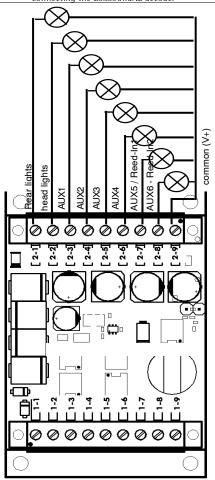
Figure 9: Connecting the LokSoundXL decoder
