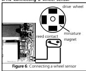
To synchronize the exhaust chuffs with the revs of the drivers an external sensor can be (but does not have to be) used. The sensor input is described in figure 6. The LokSound micro does not support this sensor input.
