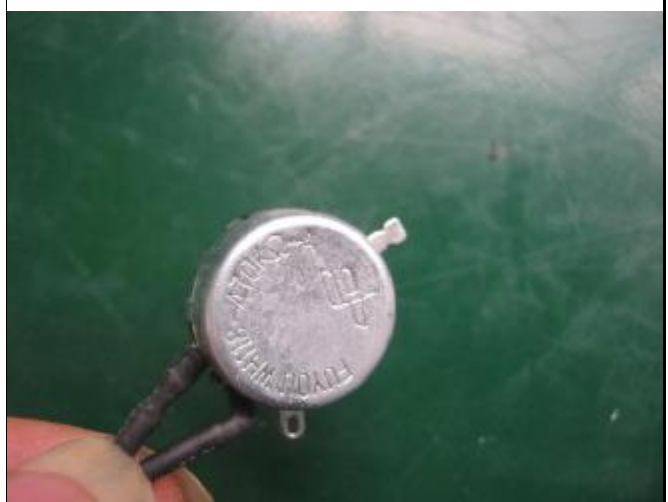
110 mark on speed adjust switch
