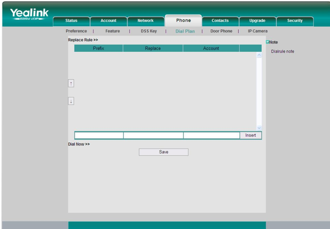
Dial-now rule: After you enable this rule, VP-2009(P) makes a call as soon as you enter the preset number. For example, if you set **Dial-now Rule** to **0147**, VP-2009(P) makes a call to 0147 for the setting time after you enter 0147. The setting time is the value which you input in the “Dial now Delay time (0~2000ms)” field. The phone supports this rule of each distinct account.
