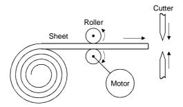
2) Turning X2 ON (Sheet feeding complete → Start cutting) X2 is turned ON the moment D0 reaches 1000. Y4 is turned OFF by turning X2 ON to stop roller operation, and cutting is executed by cutter when Y20 is turned ON.
