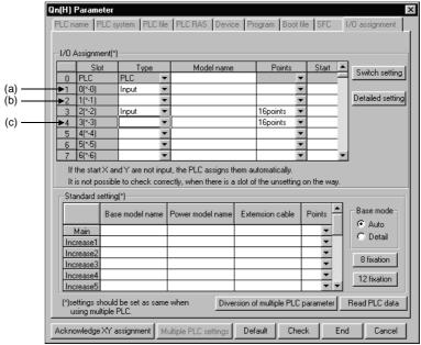
(5) Select the [Tools]  $\rightarrow$  [Start ladder logic test] GX Developer menu items to start the GX Simulator. An initial window as shown below is displayed.
