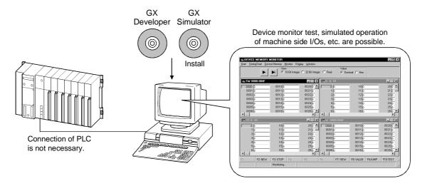
A sequence program created with GX Developer can be debugged by writing it to the GX Simulator.
