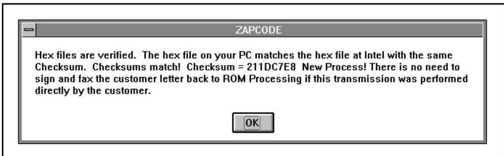
**Figure 8-13. Example of a Successful Checksum Message**
