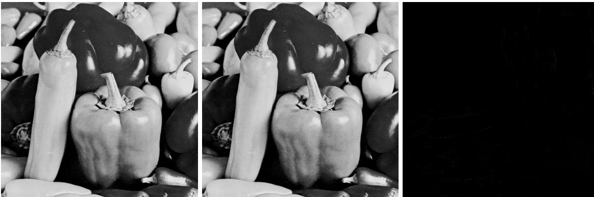
FIGURE 1. Input image (left), reconstruction (middle). The source code performs a kind of wavelet decomposition. The image on the right represents the decomposition coefficients.
