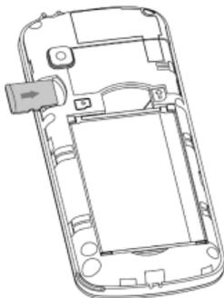
To remove the card, press and release the card so it clicks out. Then, remove it carefully from the slot.
