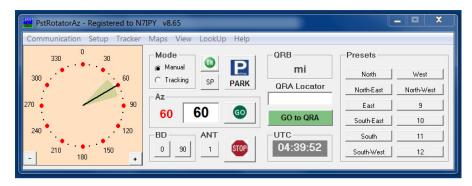
After installing the software and entering your registration code you must configure the software by setting the COM Port and Controller Type.
