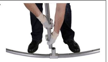
You can also place your feet on the top rails either side of the Small 'B' Socket (3) to steady the assembly, as shown in the image.
