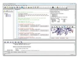
MicroSurvey STAR\*NET is an easy-to-use Windows application that adjusts 1D/2D/3D survey networks using rigorous Least Squares techniques.
