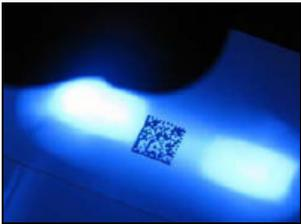
1. Hold the imager about 6" from the mark and align the blue targeting pattern as shown here.
