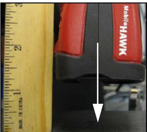
2. Move the front of the imager steadily downward toward the mark and parallel to the mark surface.
