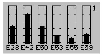
The display shows six channels on each page and there are five pages. Step through the pages with the "UP" and "DOWN" buttons.
