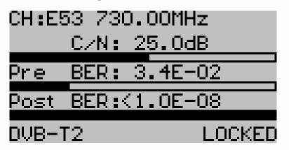
Hopefully, but not always, the digital readout; BER (bit error rate) and C/N (Carrier/Noise) will correspond well with the analog setting of the antenna.
