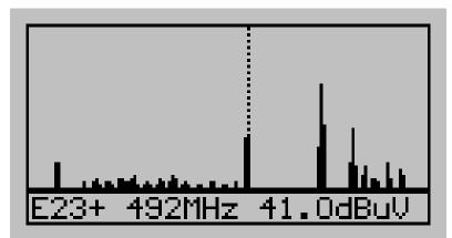
The meter shows the frequency spectrum of 48-860 MHz. A marker can select a certain channel (with the "UP", "DOWN" buttons).
