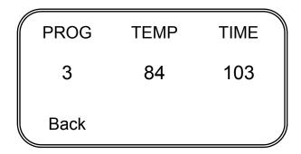
Parameters may not be altered. Press "Back" to return to the operating screen. Then if the run parameters must be altered, press "Stop" and reprogram the display as described below:
