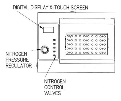
**Nitrogen Control Valves** – Used to turn nitrogen flow ON or OFF to the nozzles above the sample vials. The top valve controls the 10 nozzles on the top row. The second valve controls the second row of 10 nozzles. The third valve controls the middle row of 10 nozzles. The fourth valve controls the fourth row of 10 nozzles. The bottom valve controls the bottom row of 10 nozzles. Push the lever to the right to turn nitrogen flow ON.
