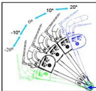
The angle adjusting gear
