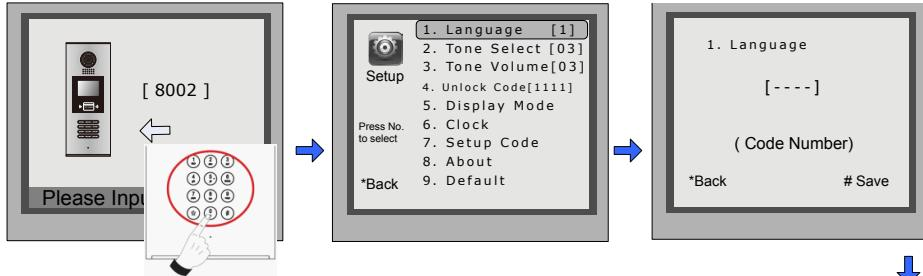
Press "#", Input "8002", then input Setup Code or Admin Code
