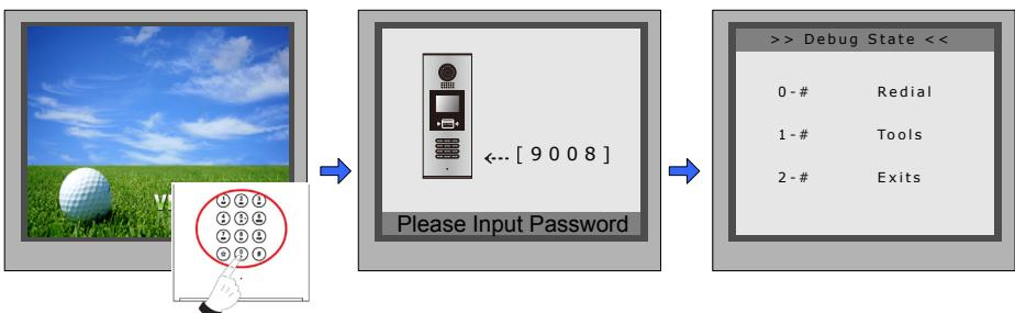
When Door Station is in standby, press '#' key
