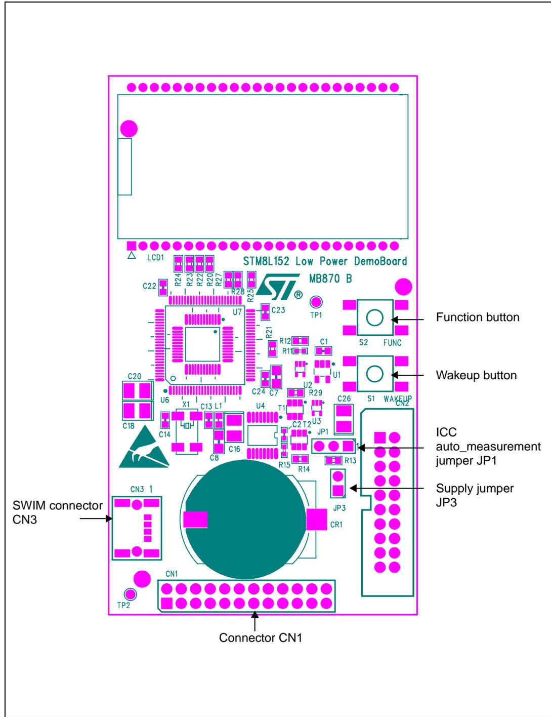
Figure 3. STM8L15LPBOARD board layout: bottom view
