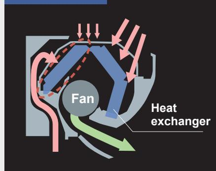
Air intake from both the top and bottom allows the back part of the heat exchanger to be used fully, resulting in higher energy efficiency.
