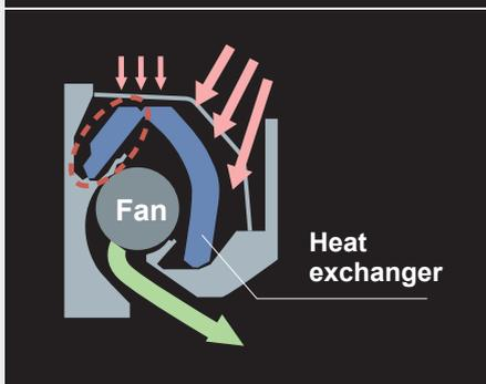
The back part of the heat exchanger is only partially used.
