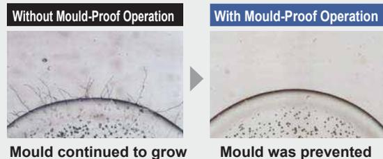
Test room: Chamber of approx. 10 m<sup>2</sup> in a laboratory at the Institute of Environmental Biology in Japan
