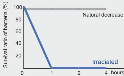
Test method: Filters were compared on a testing device with and without the streamer discharge to check their ability to adsorb mould and odour-causing bacteria.
