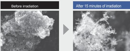
Diesel particles were placed on an electrode of the streamer discharge unit and a picture was taken using an electron microscope after 15 minutes of discharge.
