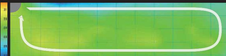
For the 5.0 kW model, the airflow distance is 12 metres<sup>2</sup>. The time required to reach the set temperature is only half of that for a conventional Daikin inverter model<sup>3</sup> for the Japanese market.
