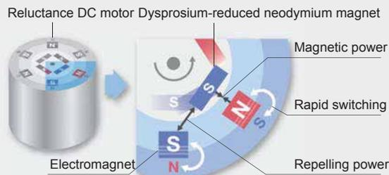
Embedding a high-strength neodymium magnet in the rotating shaft turns the entire centre of the motor into a powerful magnet. By rapidly switching the electromagnet from the N to S-pole, the Reluctance DC motor is able to produce greater speed and power. Urusara 7 uses a new dysprosium-reduced neodymium magnet.
