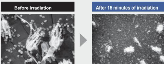
Cladosporium was placed on an electrode of the streamer discharge unit and a picture was taken using an electron microscope after 15 minutes of discharge.
