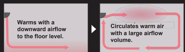
Discharges a large air volume with the Coanda mechanism.
